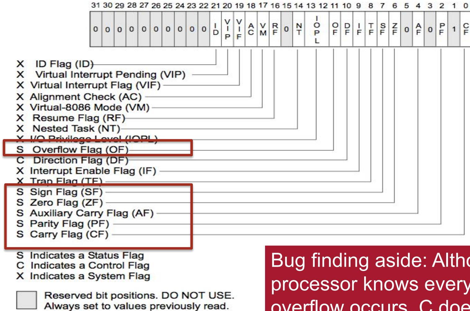
Bug finding aside: Although the x86 processor knows every time integer overflow occurs, C does not make this result visible.
